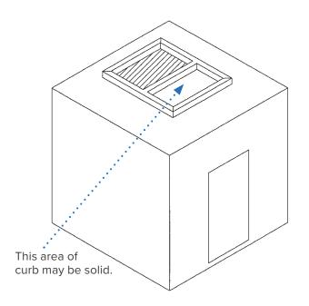
Figure 1. Curb placed on roof of walk-in cooler.
