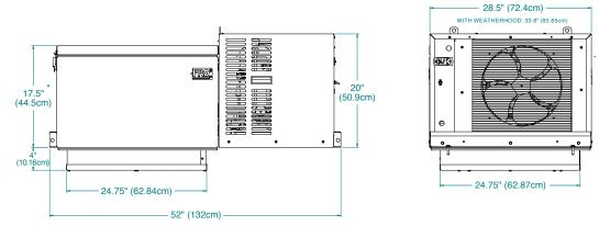
25"X25" PANEL OPENING REQUIRED FOR EVAPORATOR SECTION OF "P2" CABINET SIZES. \* - 21.5" (54.61 cm) ON OUTDOOR MODELS WITH WEATHER HOOD
