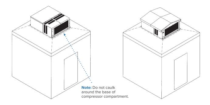
**Figure 3.** Outdoor unit placed on roof of walk-in color. (see rigging instructions).
