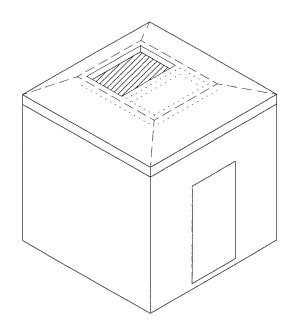
Figure 2. Roof membrane placed over curb.
