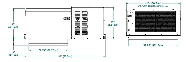
25"X38.5" PANEL OPENING REQUIRED FOR EVAPORATOR SECTION OF "P3" CABINET SIZES. \* - 23.5" (59.69 cm) ON OUTDOOR MODELS WITH WEATHER HOOD
