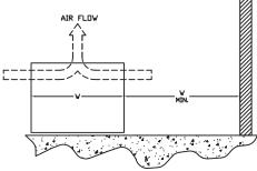
Clearance for multiple units placed side by side
