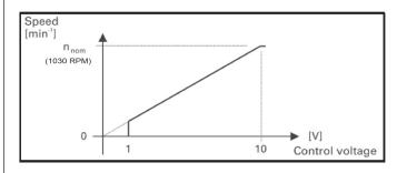
The input control signal can be supplied from any controller that outputs a 0-10 VDC signal. For units with a control signal supplied from a rack control or other external controller, the unit is provided with a terminal board for control signal wiring. Units with factory installed proportional pressure controls require no installation wiring.
