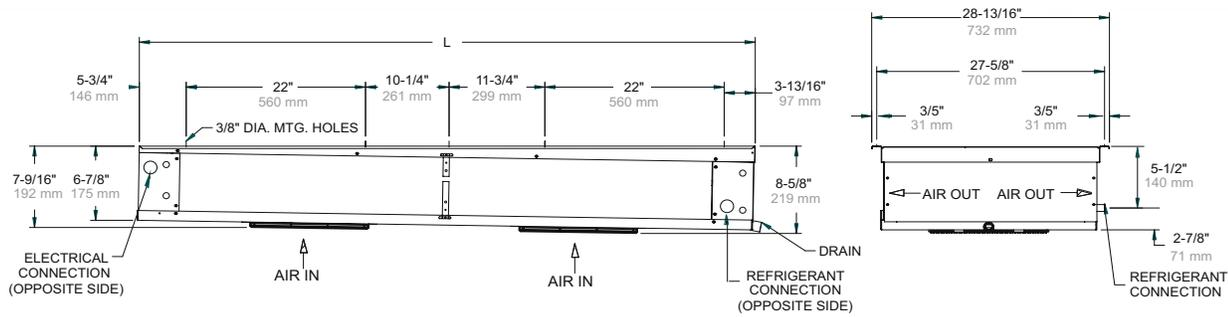
**NOTE:** All units have 1/4" OD external equalizer and 3/4" FPT drain connection
