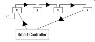
M = Master Evaporator S = Slave Evaporator CU = Condensing unit
