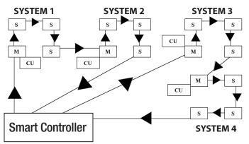
M = Master Evaporator S = Slave Evaporator CU = Condensing unit
