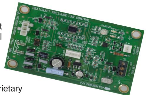
If there is a problem with the Orbus Controller, it can be disconnected and the fans will run full speed.
