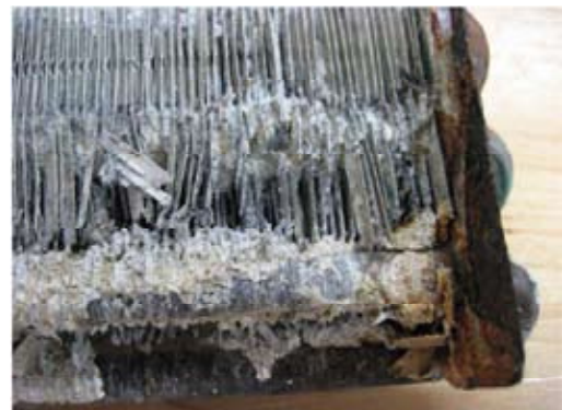
Figure 2 – RTPF Coil with 1 Year of Exposure
