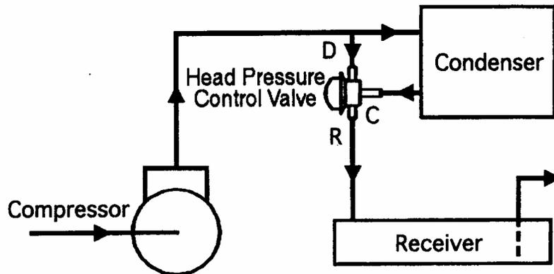
**Figure 1. Single Valve Flooded System**
