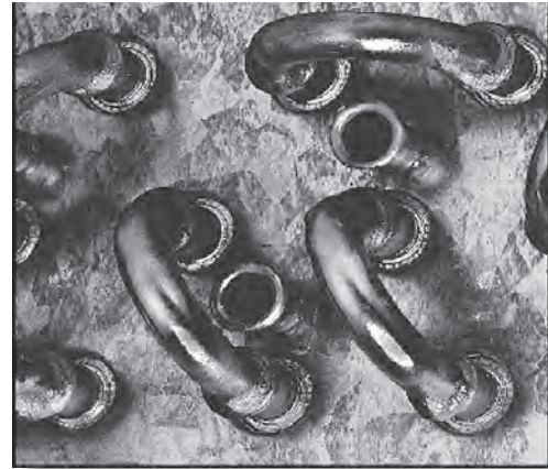
The Floating Tube Coil Design Dramatically Reduces Tube Sheet Leaks
